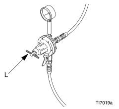
Fig. 12: Fluid Pressure Regulator
